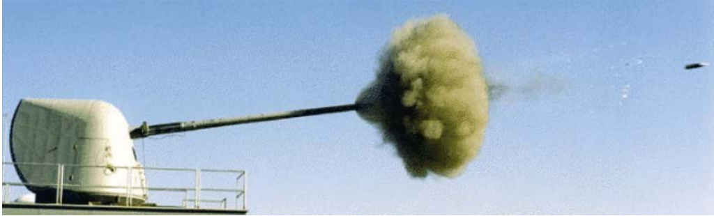
Figure 3.0-2: Gun Blast and Projectile from a 5" 54/62 Navy Gun
